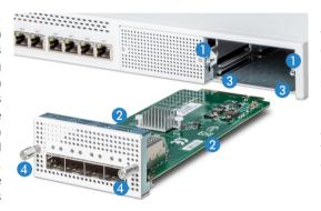
Remove the module slot cover by loosening the appropriate screws at position ①. Place the extension module in front of the module slot as shown in the illustration and push it into the slot, so that the long sides of the circuit board ② slide into the guiding rails located on the inner left and right sides of the slot ③. Push the module gently all the way into the slot. Then fasten the module to the firewall housing by tightening both screws on the frontside of the module ④.
